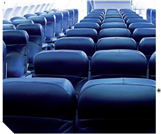
There are countless upholstery options available for airline seats, armrests and wall coverings. One form of upholstery that is becoming more popular in new and refurbished aircraft is composite leather. By using a composite leather product, airline operators could save up to 25% in fuel costs each year. Composites can be less than half the weight of natural leather.
