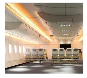
designers are given cabin elements that allow them to simulate whether things like blinds will get in the way of light from LEDs. If the simulations show a need for adjustments, the industrial design department can then adapt linings and contours to create the desired effect. Lighting designers then optimise the lights' optics. Simulations ensure the development of the bestpossible solution.
