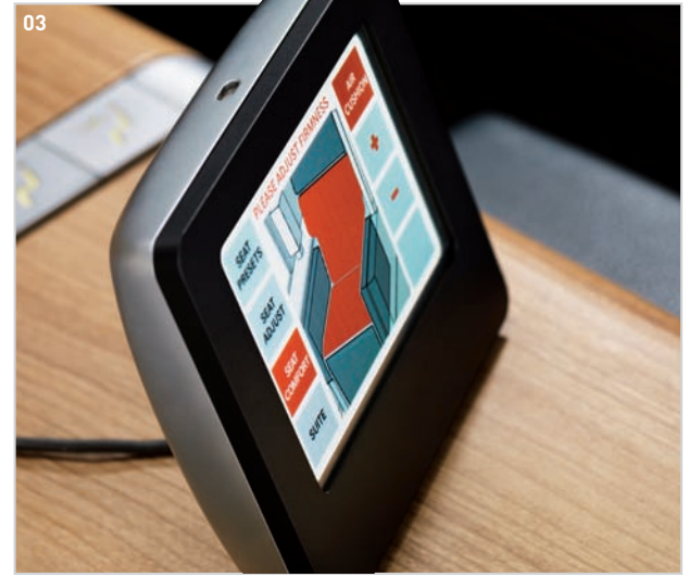
03. SWISS first-class seat control unit and GUI
