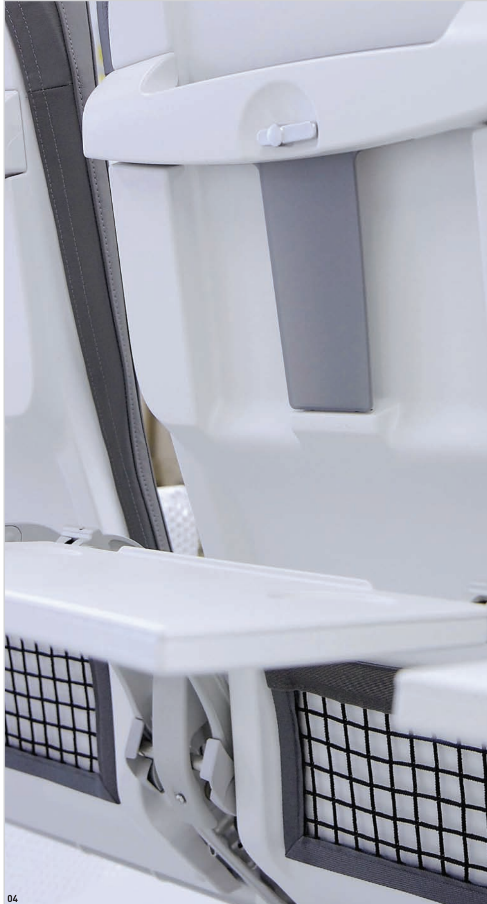
02-05. The BL3520 maximises living space with a slim backrest and the high position of its literature pocket
