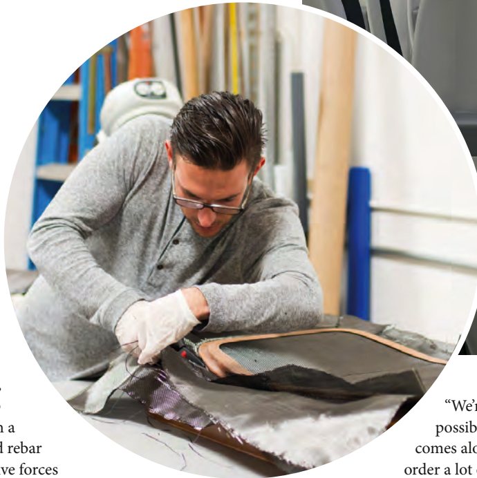
ABOVE: MUCH OF THE TOURIST CLASS SEAT IS CONSTRUCTED FROM COMPOSITES, MEANING ITS CONTOURS COULD BE SCULPTED TO REDUCE PITCH WITHOUT LOSING PASSENGER COMFORT
