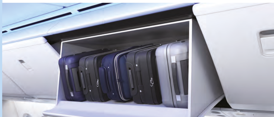
ABOVE: A FULLY LADEN STOWAGE BIN WILL REQUIRE 40% LESS FORCE TO LIFT THAN WITH THE OUTGOING B777 UNITS
