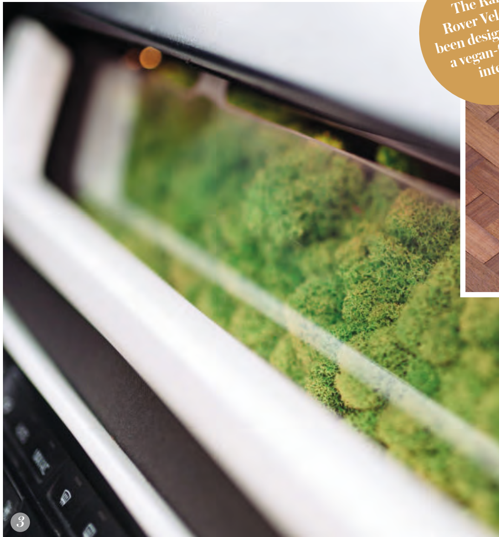
3. ICELANDIC MOSS FILTERS CABIN AIR IN THE SONO MOTORS SION
