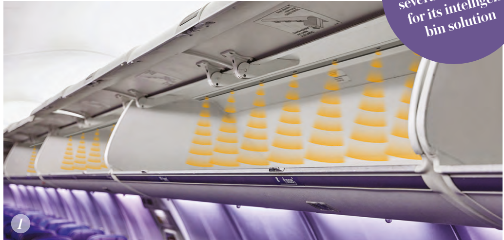
1. BIN-SENSING TECHNOLOGY ENABLES THE REMAINING OVERHEAD STOWAGE SPACE TO BE PRECISELY CALCULATED FOR CREW
