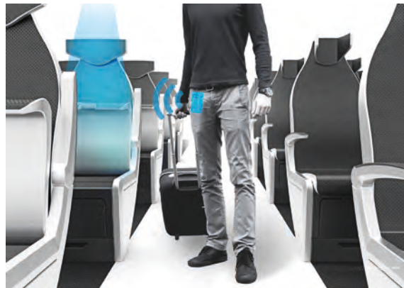
FIGURE 4 (BELOW): AS THE TICKET HOLDER GETS CLOSER TO THE SEAT, THE LIGHT BECOMES BRIGHTER (DESIGN: S AKKERMAN)
