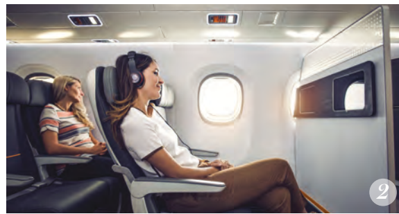
1+2. THE E2 CABIN FEATURES INDIVIDUAL OVERHEAD CONTROLS AND 90% MORE STOWAGE SPACE THAN THE FIRST E-JETS
