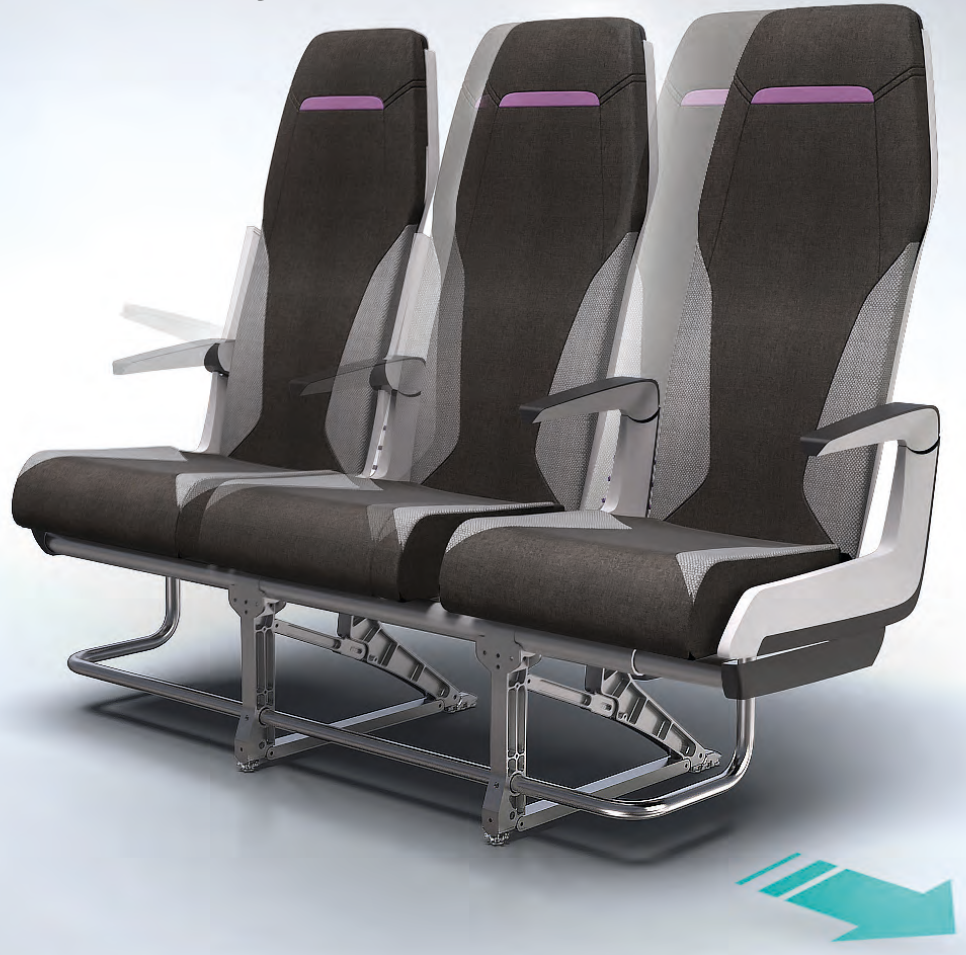
FIGURES 5 AND 6 (ABOVE AND ABOVE LEFT): THE PASSENGER SEATS CAN BE NARROWED TO WIDEN THE AISLE DURING BOARDING, AND EXPANDED AGAIN AFTER BOARDING HAS BEEN COMPLETED
