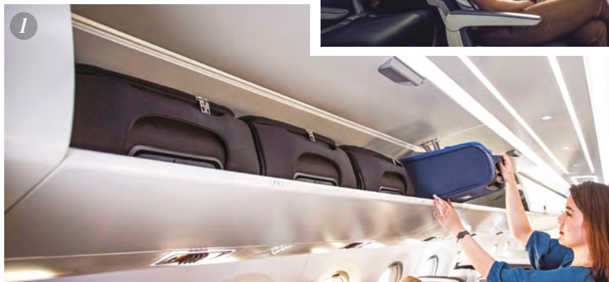
1+2. THE E2 CABIN FEATURES INDIVIDUAL OVERHEAD CONTROLS AND 90% MORE STOWAGE SPACE THAN THE FIRST E-JETS
