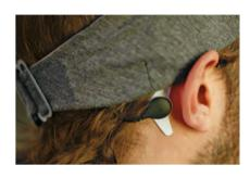
responding with tones if they are ready for a boost. An algorithm customizes the timing and volume of tones to boost slow waves, to make the most of deep sleep.
