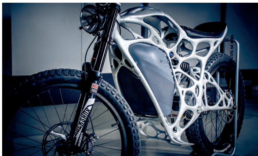
BELOW: AIRBUS SUBSIDIARY APWORKS 3D PRINTED THIS MOTORCYCLE, CLAIMED TO BE 30% LIGHTER THAN AN EQUIVALENT CONVENTIONAL MACHINE
