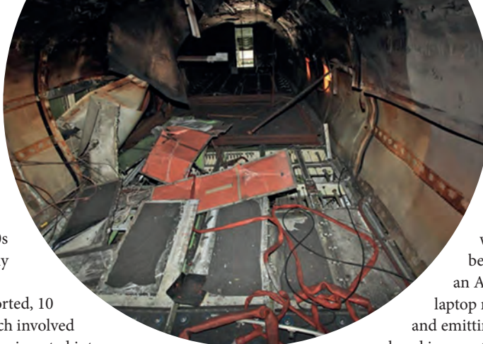
IN THIS 2013 FAA TEST, A SINGLE LITHIUM METAL CELL IN THERMAL RUNAWAY LED TO A FLASH FIRE, AND A HUGE EXPLOSION WHEN MIXED WITH FUMES
