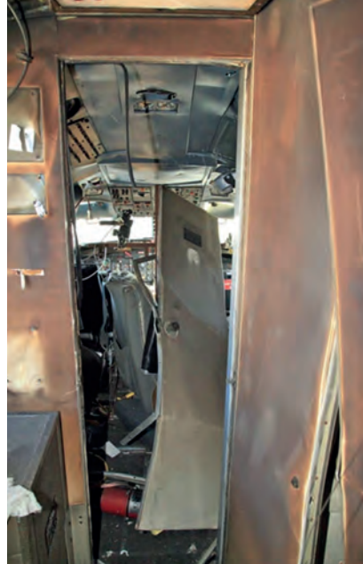
DURING AN FAA TEST, A SINGLE LITHIUM CELL IN THE HOLD HELPED CREATED A BLAST STRONG ENOUGH TO BLOW THE COCKPIT DOOR OFF ITS HINGES
